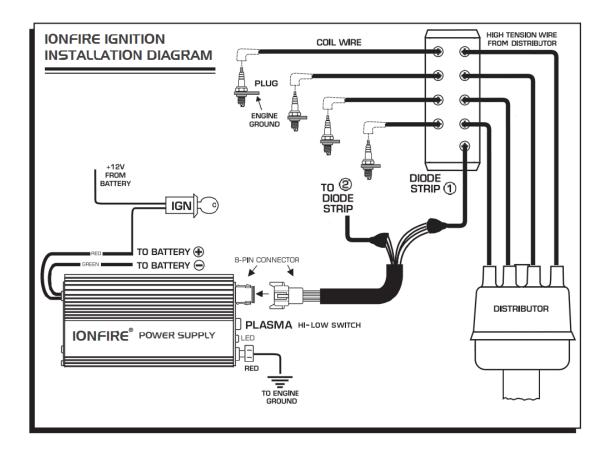
5. Connect the 12 VDC power supply cables of the plasma Ignition module to the vehicles battery or a 12VDC supply
